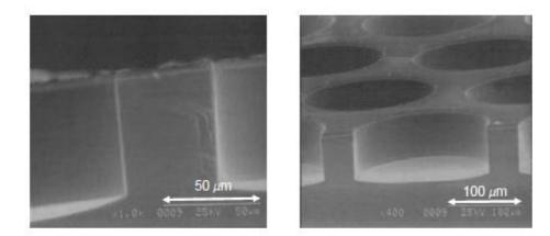
Etch Rate: ~7um/min for 1:2 Aspect ratio and PR passivation. ~10um/min for very open area with no PR passivation. Selectivity with PR: ~10:1 for via holes Selectivity with SiO2: ~90:1 for low aspect ratio open areas
