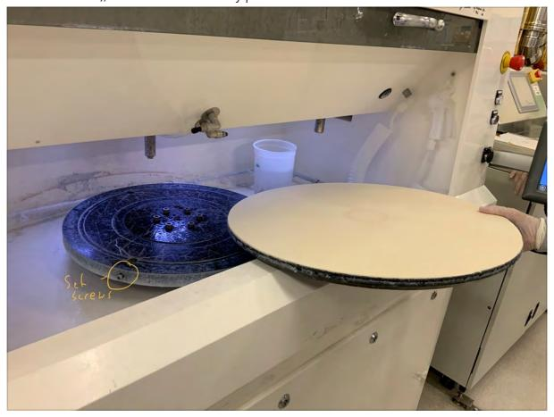
On display once all lights are green can run in manual mode or use recipe choose which water pump you want to use (1 to 2) then put the corresponding two hoses in the slurry container (take them out of the water bucket)
