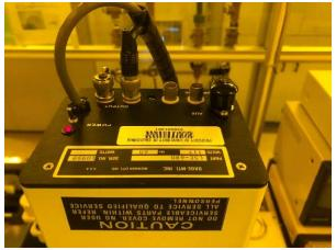
5. Open the small panel on the front of the IR camera monitor and move the POWER switch to the ON position, it will take ~30 seconds to warm up.
