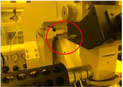
**NOTE:** The MICROSCOPE ILLUMINATION knob is used for adjusting topside alignment light output (visible light, viewed through the eyepieces).
