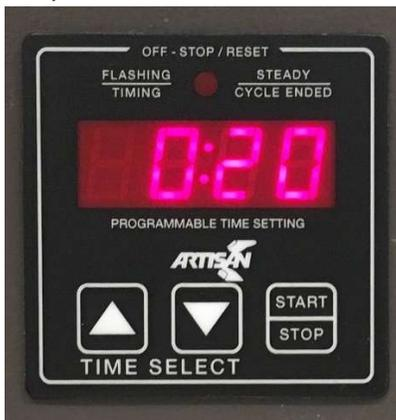
15. Press the START/STOP button to start the timer and turn on the RF power. The green RF ON LED on the RF power supply should illuminate.
