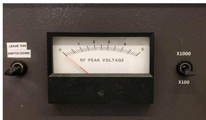
**NOTE:** The multiplier switch next to the meter adjusts the scale of the meter, in most cases X100 is adequate.
