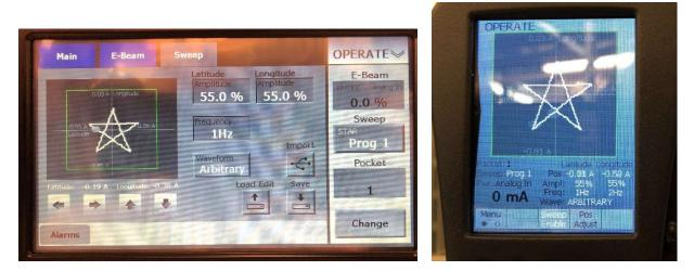
h. You are allowed to adjust the sweep parameters (size, shape, frequency and position), but you are not allowed to save your changes when you are finished. As soon as you make any change to a sweep program, both the handheld and EBC screens will read Editing. After your run is completed or if you decide to change the program, <u>ALWAYS</u> <u>select Exit Edit</u> to ensure the changes you made were not saved to the program.
