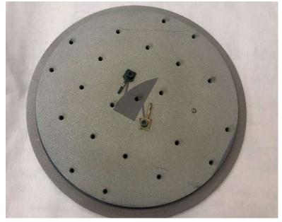
For the heated holder, mount your samples or full wafer on the supplied TOX wafer. Use the 1/16 Allen wrench/driver to loosen the Inconel clip screws and always use the blue handle torque driver to tighten them. The Inconel sample clips must be in all 8 positions as pictured below.
