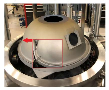
Place a 75 x 50 mm glass slide, standing on its shorter edge, on the front of the dome tooling (these are the larger glass slides in the lab). THIS IS VERY IMPORTANT AS
