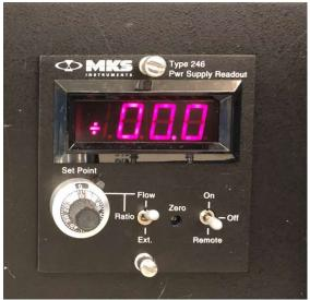
Move the other switch up to the On position and begin to introduce gas into the chamber by slowly turning the Set Point dial clockwise. When introducing gas into the chamber do it in increments of 5 SCCM at a time, waiting for the chamber pressure reading on the ion gauge chamber gauge to drop or stabilize each time before proceeding.
