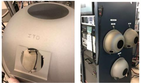
• Carefully re-install the dome tooling, making sure to insert the O2 gas line into its hole.
