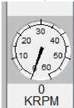
6. Once the spindle has reached 0 RPM; close the spindle cover and lock, remove the interlock key and close the dicing saw cover fully.
