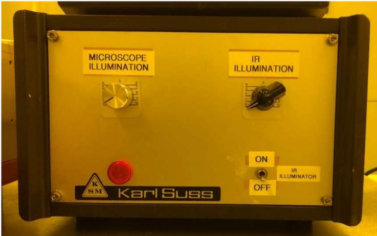
10. Use the IR ILLUMINATION knob to adjust the IR ILLUMINATOR light output to the desired level.
