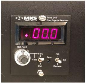
18. Move the other switch up to the On position and begin to introduce gas into the chamber by slowly turning the Set Point dial clockwise. When introducing gas into the chamber do it in increments of 5 SCCM at a time, waiting for the chamber pressure reading on the chamber gauge to drop or stabilize each time before proceeding.
