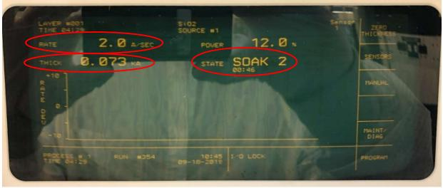
The image below shows rate and thickness readings during the Soak 2 step.
