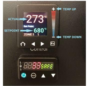
**IMPORTANT:** The setting you set the heater to is not what the sample temperature will be, you will need to reference the **Temperature Offset Table.**
