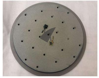
• For the heated holder, mount your samples <u>or full wafer</u> on the supplied TOX wafer. **Use** the 1/16 Allen wrench/driver to loosen the Inconel clip screws and always use the blue handle torque driver to tighten them. The Inconel sample clips must be in <u>all 8</u> positions as pictured below.
