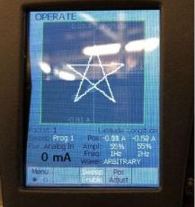
h. You are allowed to adjust the sweep parameters (size, shape, frequency and position), but you are not allowed to save your changes when you are finished. As soon as you make any change to a sweep program, both the handheld and EBC screens will read Editing. After your run is completed or if you decide to change the program, <u>ALWAYS</u> <u>select Exit Edit</u> to ensure the changes you made were not saved to the program.
