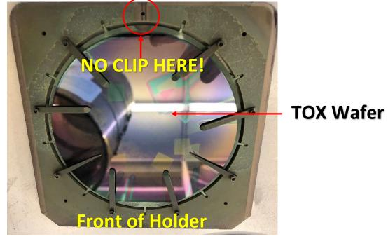
**IMPORTANT:** There is a 9<sup>th</sup> clip position circled in red above. DO NOT place a clip in this position as is will interfere with the thermocouple contact and damage it!
