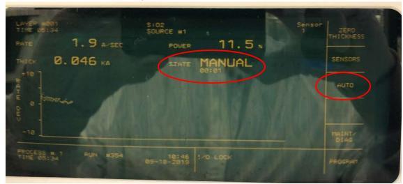
j. You can now control the power using the hand-held controller. Slide the switch on the top of the controller to the left (INCR) to increase the power and to the right (DECR) to decrease the power. Take care not to press down (STOP) on the switch as that will stop the deposition process.
