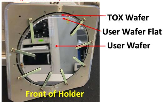
**IMPORTANT:** When running a full 4" wafer, the wafer must be mounted as follows or else damage to the thermocouple will occur!
