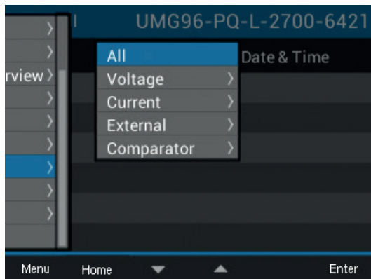
Fig. Submenu for displaying recorded events
