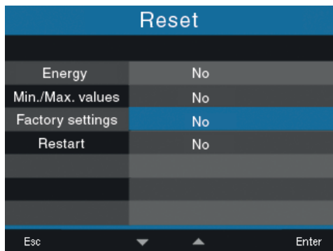
Fig. Reset window, standard factory settings
